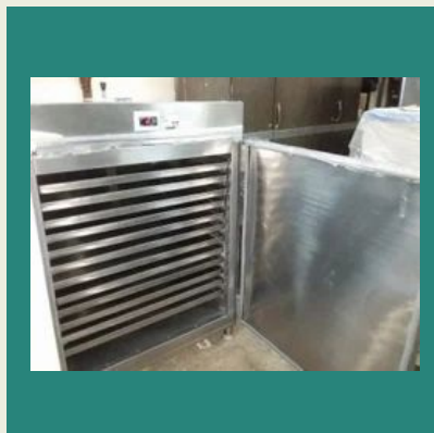
Vegetable Dehydration Plant
